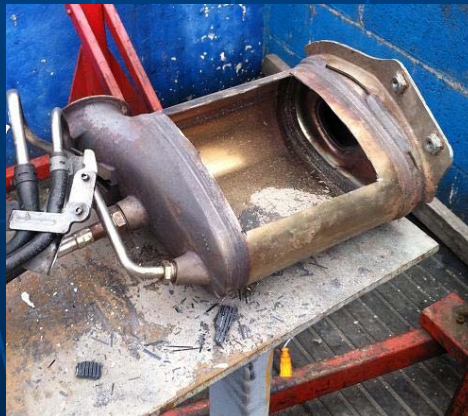
The DPF filter once The contents have been removed.
