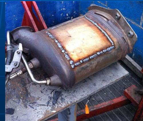
The DPF Filter re-welded to be re-fitted.
